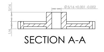
Part Number: PLASTOCK ® 24-60 Manufactured by Putnam Precision Molding Part Description: www.plastock.biz Delrin Spur Gears 24 Pitch - 20° Pressure Angle © 2010 Putnam Precision Molding Dimensions are in inches Tolerances: PROPRIETARY AND CONFIDENTIAL : THE INFORMATION CONTAINED IN THIS DRAWING IS THE SOLE PROPERTY OF PUTNAM PRECISION MOLDING. MOLDING IS PROHIBITED. INFORMATION IN THIS DRAWING IS PROVIDED FOR REFERENCE ONLY. Unless Explicitly Stated Assume  $\pm 0.015$
